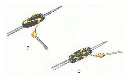
Fig. 15. How the beads are made
