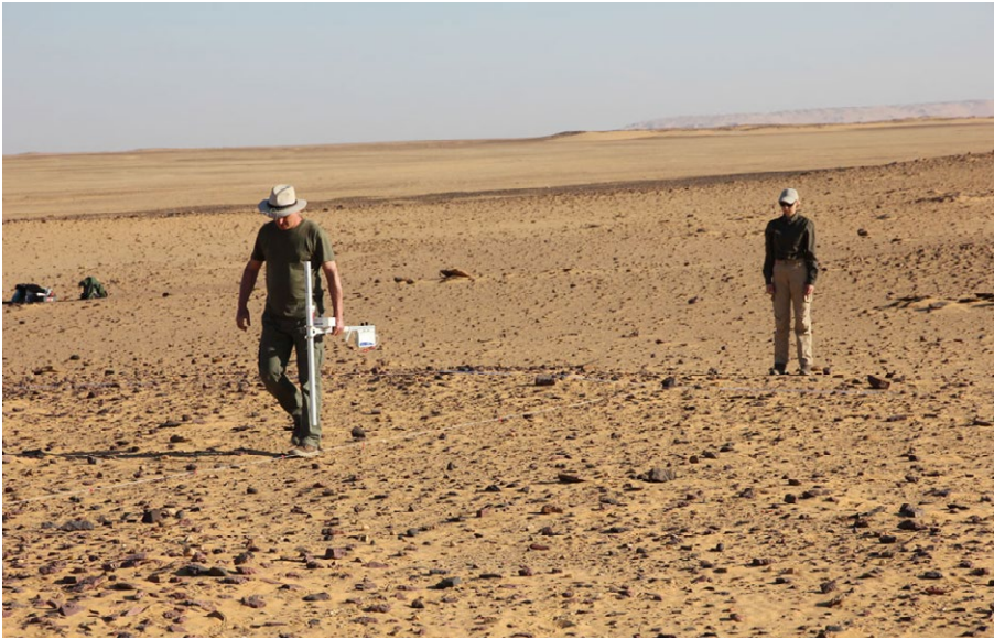
Fig. 4. At Bargat El-Shab, gradiometer data was collected using the Bartington Grad 601 gradiometer with single sensor placed close to the ground (approx. 20 cm above the surface). Photo: P. Bobrowski.
