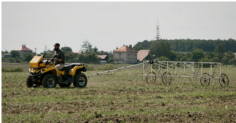
Fig. 7. Magnetometer measurement at the location of fortified point No. 3. Photo: P. Vrba.
