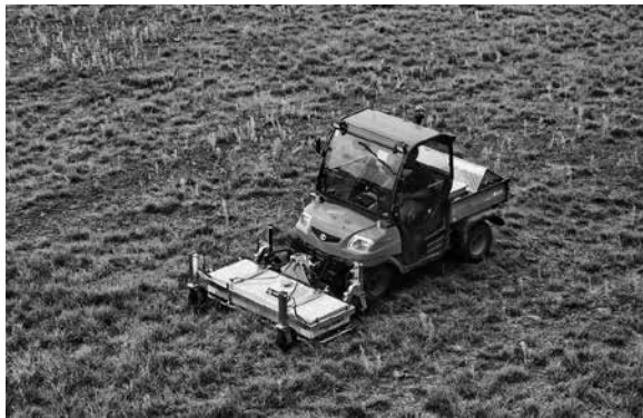
Fig. 2. MALÅ MIRA 16-channel GPR system in adapted version for the prospection of the Roman town of Carnuntum
