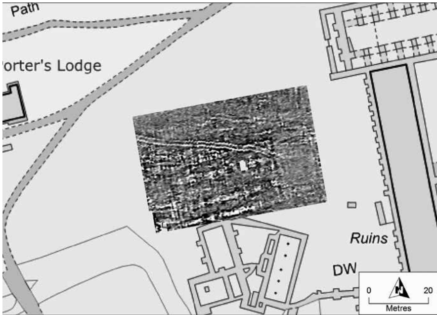
Fig. 3. Earth resistance results using an a=0.75 m square array in gamma configuration. Data were interpolated, displayed from 1.5 SD (white [low] – high [black])
