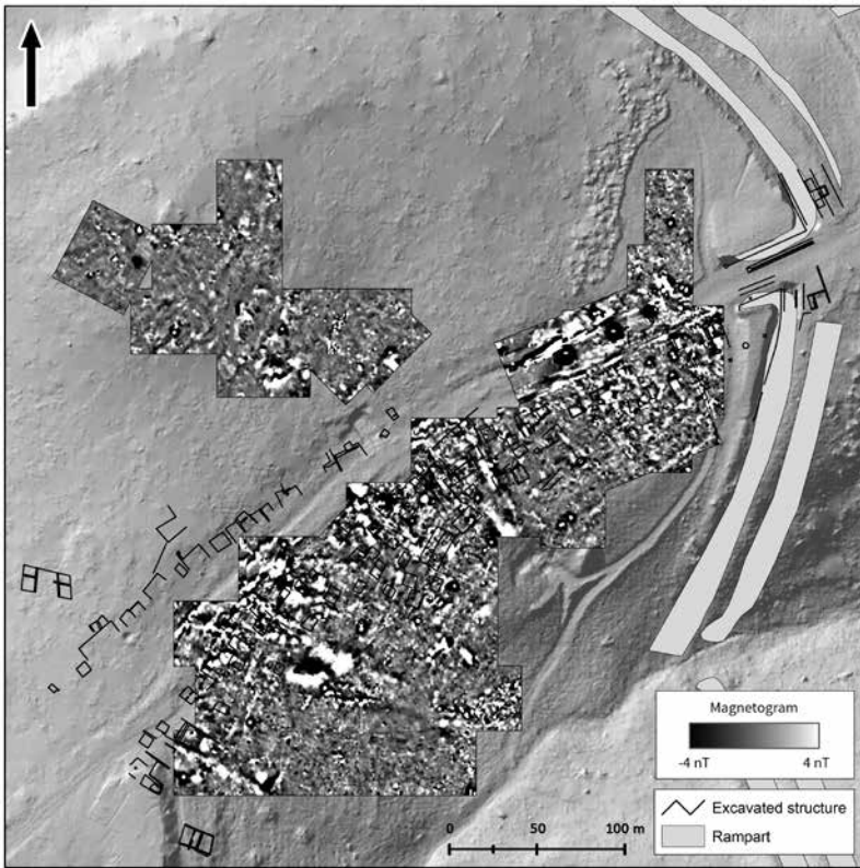
Fig. 2. Bibracte, Côte Chaudron. Magnetic map (raster 0.25 m/0.50 m, dynamics of measured values -4/+4 nT in 256 shades of grey: black/white) overlaid by the plan of earlier archaeological excavation
