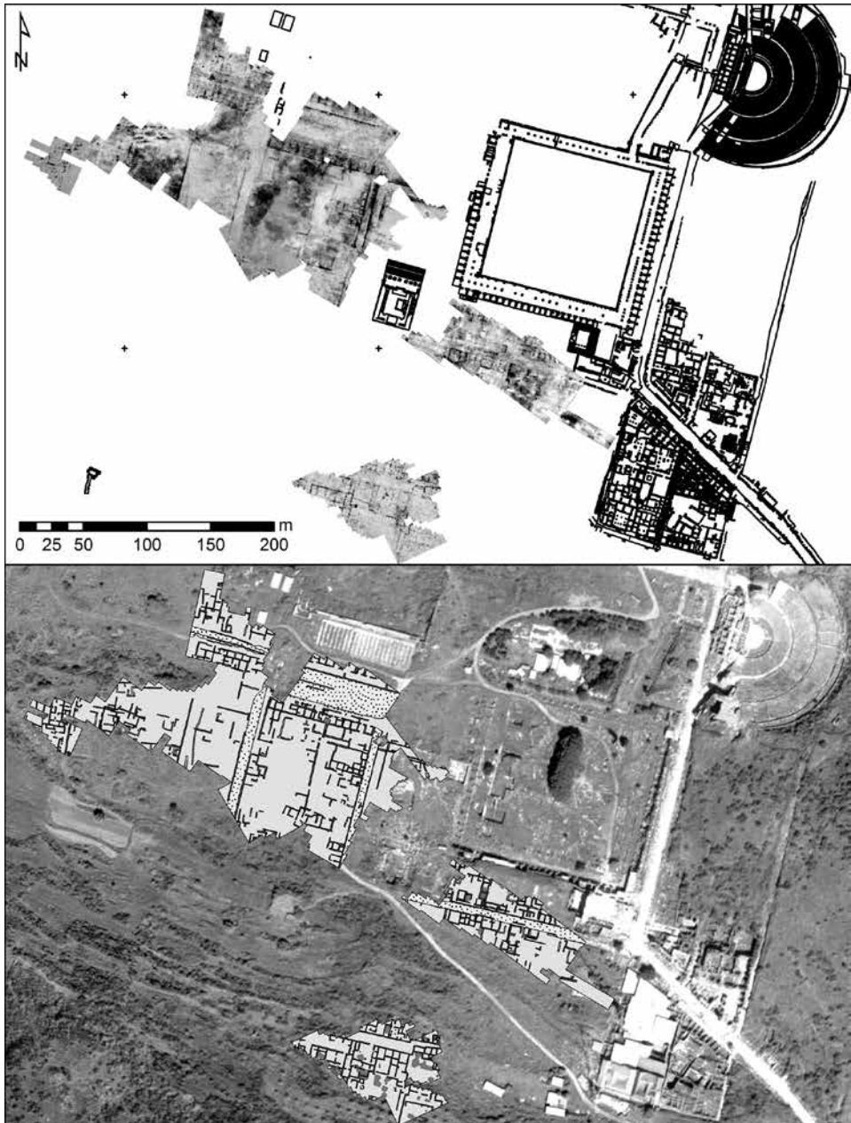
Fig. 3. The results of GPR prospection in the area of the Serapeion in Ephesos above (black: high amplitudes – reflective, white: low amplitudes – absorbent) and the archaeological interpretation below
