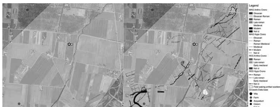
Fig. 2. The Rusellae/Grosseto study area. Left. Part of the sample transect with red to show the results of traditional archaeological survey. Right. The same area showing integrated remote sensing survey and GIS-based data mapping. Grey scale mapping drawings show the various kinds of natural and archaeological features identified so far. The quantitative and qualitative improvement in the landscape database is clearly visible, making it possible to ask, and eventually to answer, new archaeological questions about field systems, communication routes, settlement patterns, and former water courses that may have conditioned settlement and land-use within the sample area. The smaller-scale inset in the top left corner of the diagram shows the areas of completed geophysical prospection in dark grey, clearly demonstrating the correspondence between detected features and the adopted survey method
