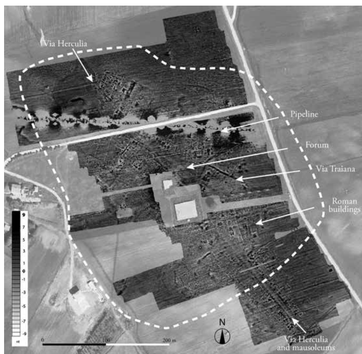
Fig. 3. Results of a geophysical magnetic survey performed in the area of Aequum Tuticum
