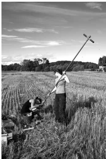
Fig. 1. Using a liner sampler to evaluate the interpretations of GPR and magnetic data sets
