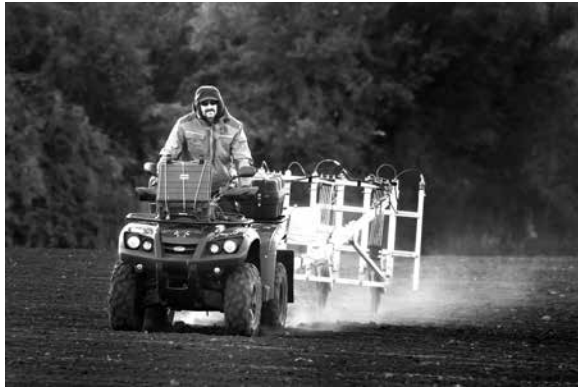
Fig. 1. Motorised 8-channel fluxgate magnetometer system used for the magnetic survey of Carnuntum
