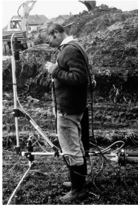
Fig. 18. Helmut Becker using a Varian V101 caesium magnetometer in gradiometer mode. Survey in Aiterhofen, Lower Bavaria, in 1979. Archive of Jörg Fassbinder
