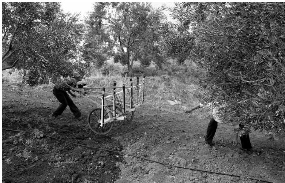
Fig. 1. The LEA MAX magnetic gradiometer array in the olive groves at Yeni Yeldeğirmentepe
