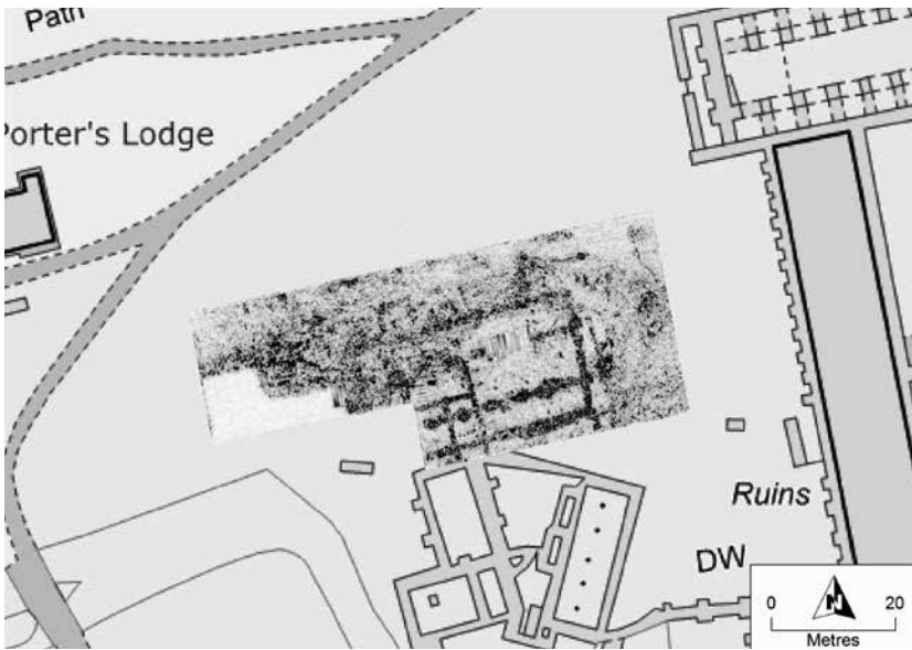
Fig. 2. GPR time slice correlating to a depth of 1.67 m (white [low] – high [black])
