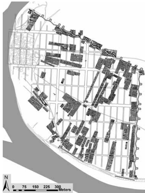
Fig. 3. Example of orthogonal city planning: magnetic map on the site of Apamea on the Euphrates (Turkey) (scale white/black -10/+10 nT/m)
