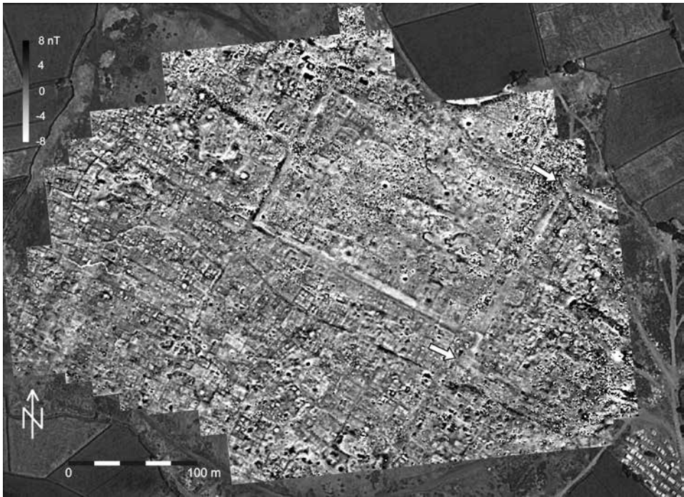
Fig. 4. Kom el-Gir. Magnetic map of Roman-period architecture. Arrows point to anomalies that reflect the position of the northern and western corners of a hypothetical fort. Satellite image by Google Earth
