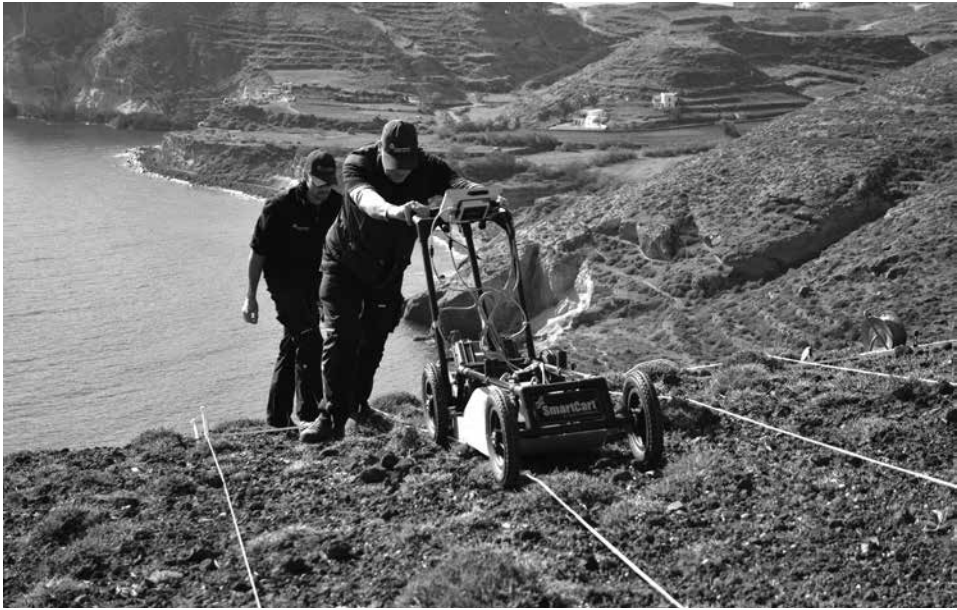
Fig. 1. Ground penetrating radar measurements with a 250 MHz antenna system and 25 cm profile spacing on top of Kokkino Vouno (Red Mountain) near the archaeological site of Akrotiri. Photo: LBI ArchPro, Klaus Löcker
