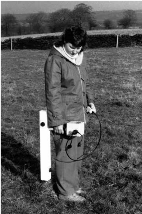
Fig. 17. Kath Walker of Geoscan Research with a prototype of a FM36 fluxgate gradiometer, 1986. Archive of Geoscan Research
