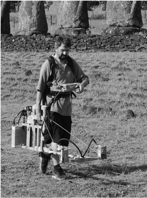
Fig. 25. Jörg Fassbinder taking measurements on Easter Island, using Smartmag SM4G caesium magnetometers by Scintrex, Canada. Archive of J. Fassbinder
