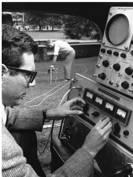
Fig. 6. Irwin Scollar taking test measurements in a park in Bonn with the first ever digital differential proton magnetometer, which he and his technician, Merken, custom-built to his design in the Rheinisches Landesmuseum in Bonn in 1960. Archive of the Ludwig Boltzmann Institute for Archaeological Prospection and Virtual Archaeology
