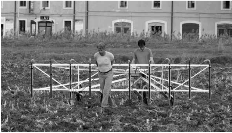
Fig. 2. Magnetic survey at Ad Medias using the LEA MAX with 10 gradiometer probes; four individual suspended wheels reduce the effect of the heavily ploughed fields
