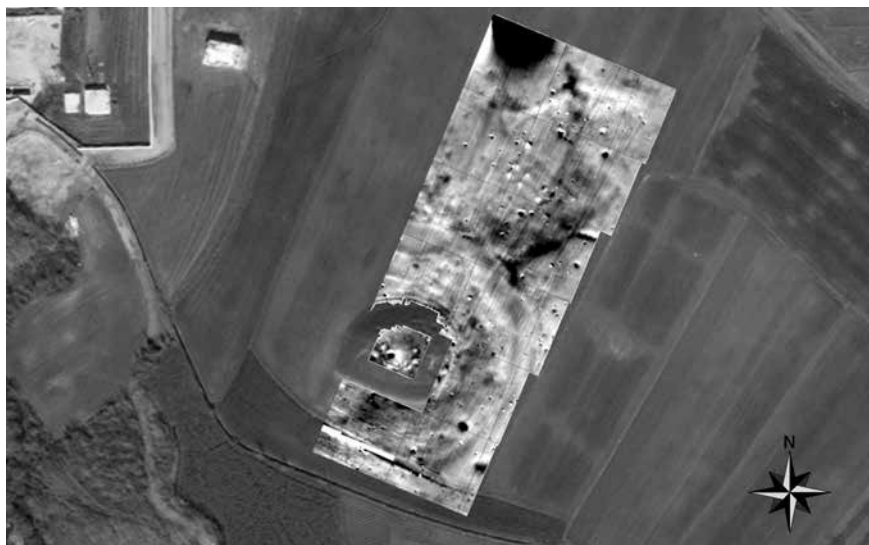
Fig. 3. Tell Kazhaw. Aerial image fused with magnetic data. Caesium-magnetometer Scintrex, Smartmag SM4G-Special, dynamics \pm 10 nT in 256 greyscales, sampling rate interpolated to 25 x 25 cm, 40 m grid
