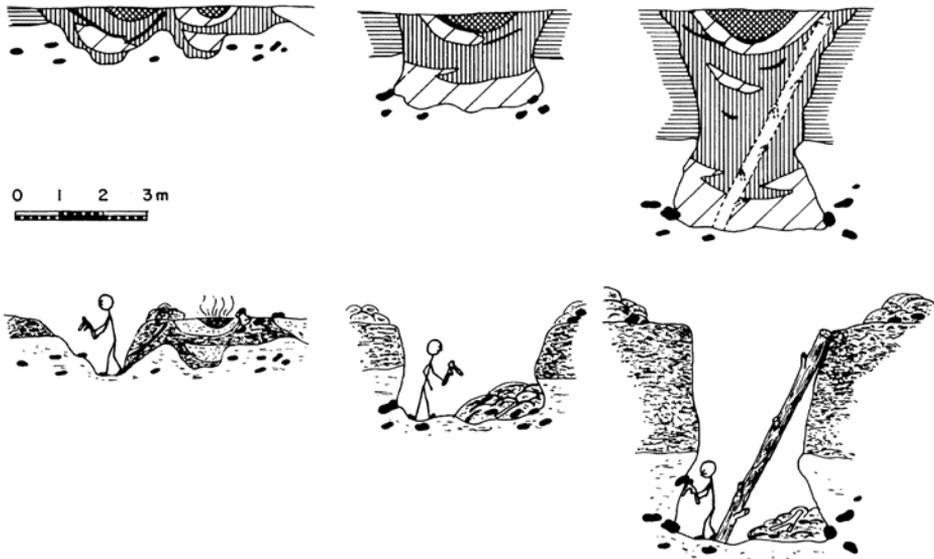
Fig. 3. A generalised sketch of the various types of flint mines at Södra Sallerup. The shallow open-cast pit type is shown to the left, the medium-sized type in the middle and the deeper mine shaft type to the right. Illustration: Elisabeth Rudebeck, Sydsvensk Arkeologi.
