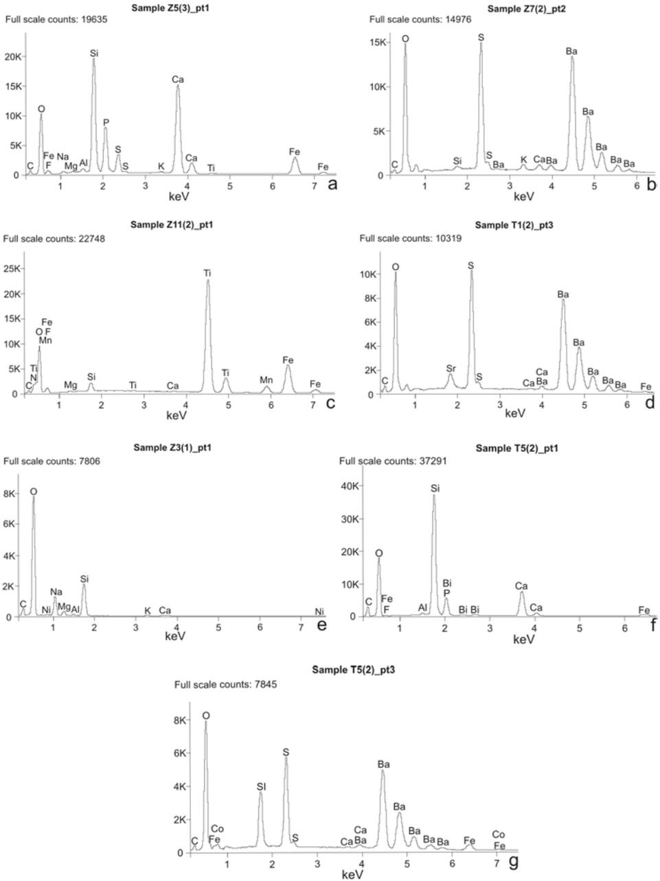
Fig. 5. EDS spectra of selected samples of Zawada flint (a–c, e) and artifacts (“T” samples) from site 6 in Tominy (d, f–g). Prepared by: M. Huber.
