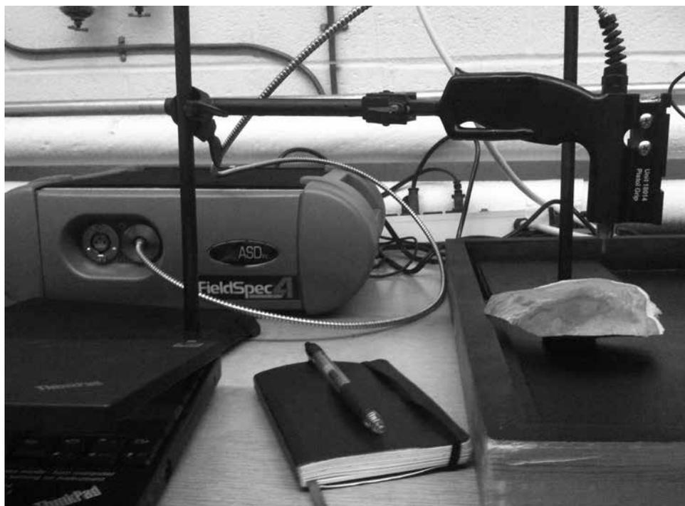
Fig. 3. An ASD Inc. FieldSpec<sup>®</sup> spectrometer used to obtain spectra in the visible and near-infrared regions. Photo: R.M. Parish.
