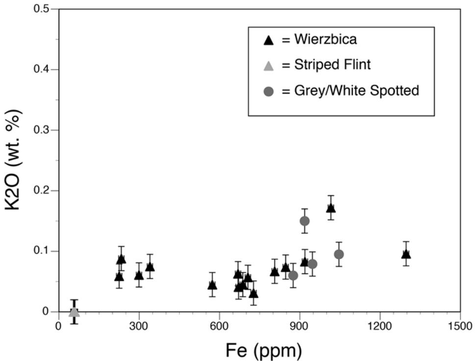
Fig. 4. The composition of K<sub>2</sub>O vs. Fe in 'chocolate' flint from Wierzbica quarry and Wierzbica 'Zełe' mine compared with geological samples of Gray-white spotted and Striped Flint. Error bars delimit 95% probability estimates for elemental composition. Graphic design: R.E. Hughes.
