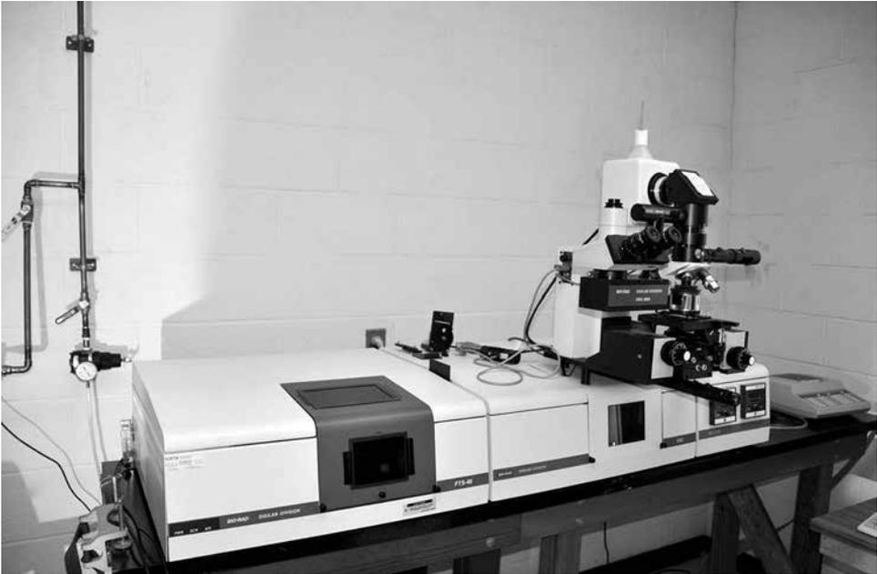
Fig. 4. A BioRad FTS-40 FTIR spectrometer used to obtain spectra in the middle infrared region.
