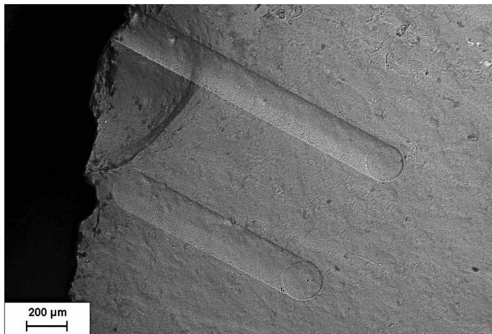
Fig. 3. The surface of sample K\_1 with a visible ablated area. Photo: G. Szczepańska.
