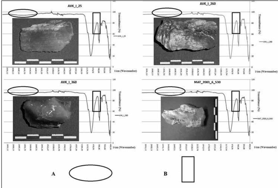
Fig. 4. IR spectroscopy diagrams: A. The decreasing of water content in the Avas-type limnosilicite (Typ 1.) samples; B. Recrystallization of the amorphous SiO<sub>2</sub>. Graphic design: Henrik Zoltán Tóth.
