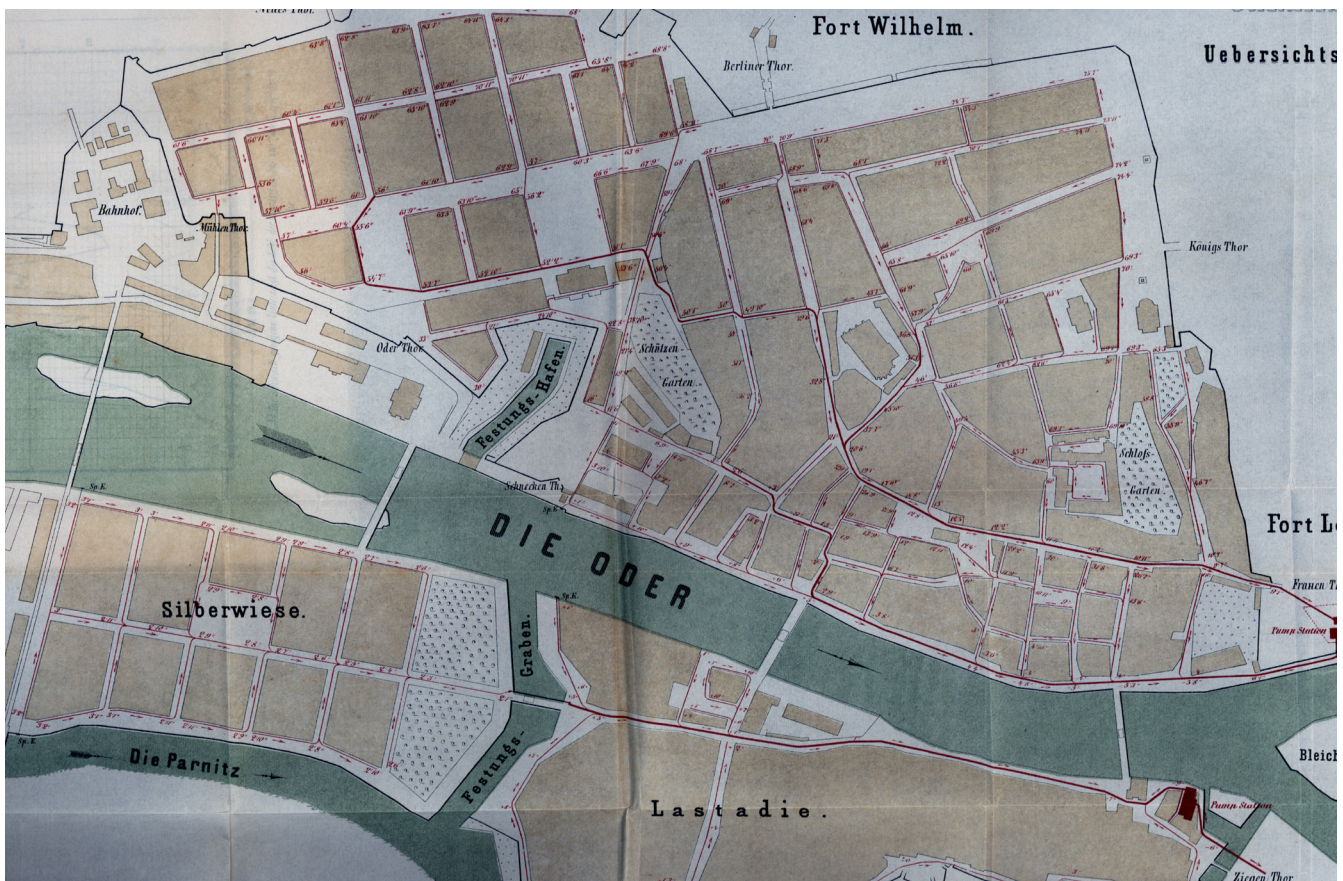
Fig. 2. Drainage project of Szczecin developed by J. Hobrecht. After Hobrecht 1868, Plan no. 2.
