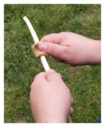
Fig. 5. Arrow shaft plane at work. Photo A. Ginter.
