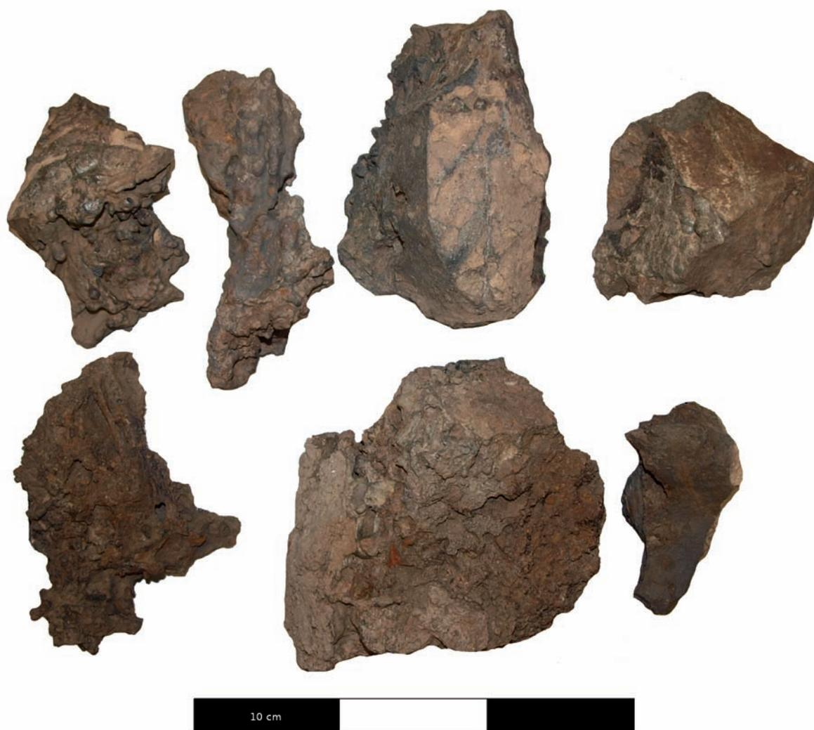
Fig 22. Pielgrzymowice 5. Trench 3. Smelting slag from furnace (feat. 1/3) (photo E. Lehnhardt)
