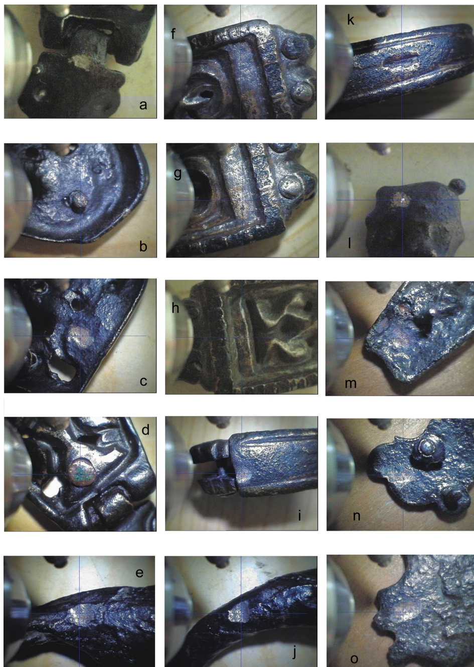
Fig. 6. Selected places of metallographic analyses: CL20883 (a-d); CL20884 (f-i,k); CL20885 (e); CL20886 (j); CL20887 (l); CL20891 (m); CL20892 (n); CL20893 (o). Photo P. Gan
