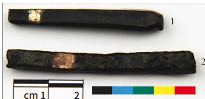
Fig. 7. Bars of raw material cleaned of patina at the measurement points with visible colour differentiation: CL20922 – multi-component alloy CuZnSnPb (a), CL20923 – tin-lead bronze alloy (b). Photo P. Gan
