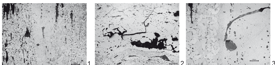
Fig. 10. Structural composition of the Żelechów hackbut: 1 – middle section; 2 – transition zone between the outer casing and the 'core'; 3 – internal section. Photo: Z. Hensel
