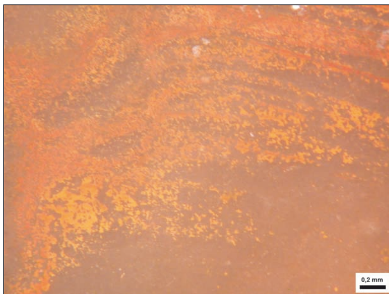
Fig. 7. Micro-cracks in the brown silicite are covered by Fe-compounds. It is evidence of the original occurrence of nodules in red clays, products of intensive weathering of probably Jurassic limestone. Investigated in water immersion under a stereomicroscope. Photo by A. Přichystal
