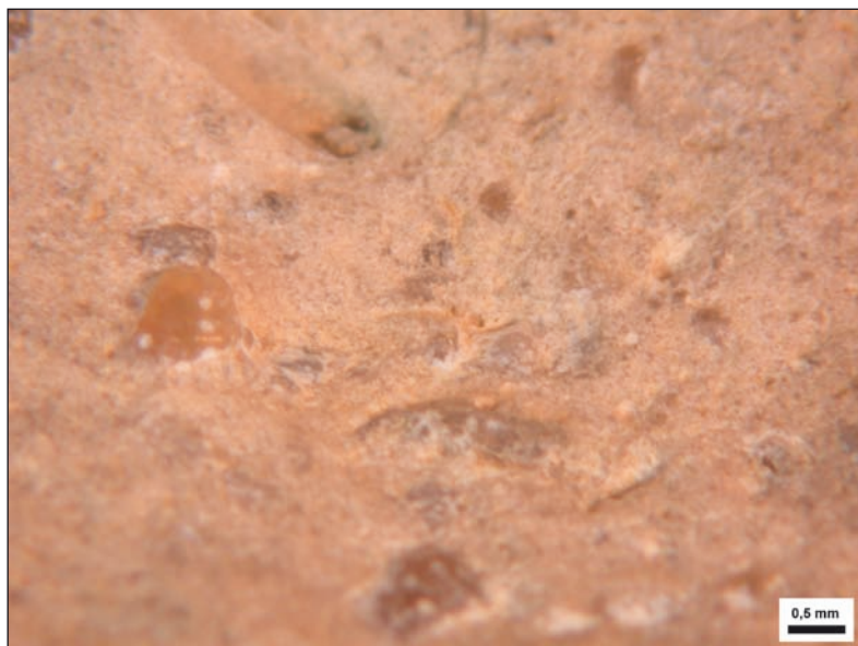
Fig. 4. Detail of the surface with small hard overgrowths. Photo by A. Přichystal
