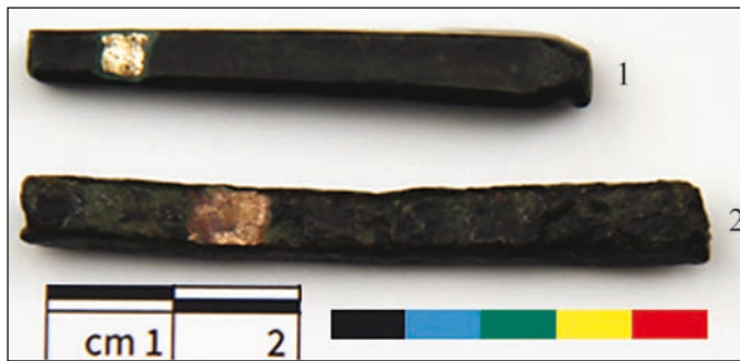
Fig. 7. Bars of raw material cleaned of patina at the measurement points with visible colour differentiation: CL20922 – multi-component alloy CuZnSnPb (a), CL20923 – tin-lead bronze alloy (b). Photo P. Gan
